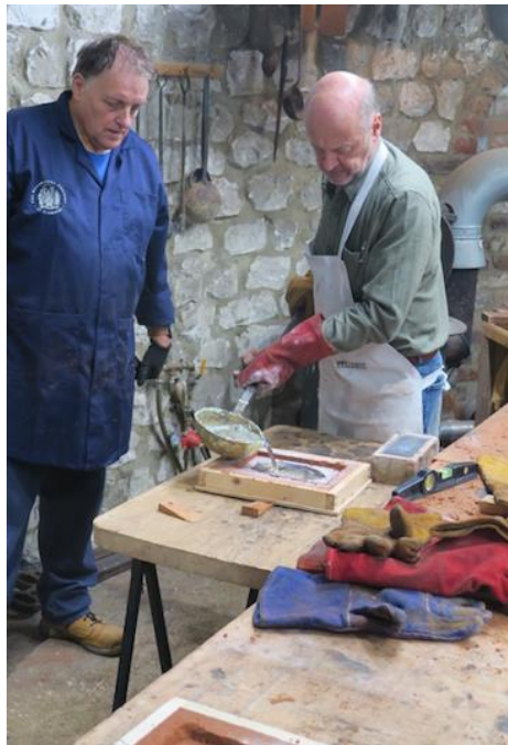
Pouring molten lead into the mould
