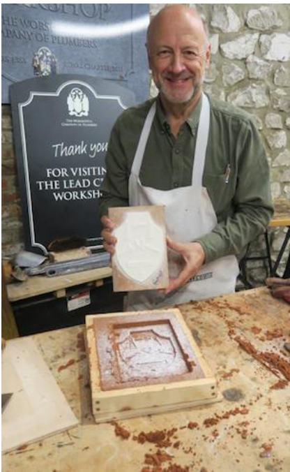
The Plumber's Shield mould ready for casting
