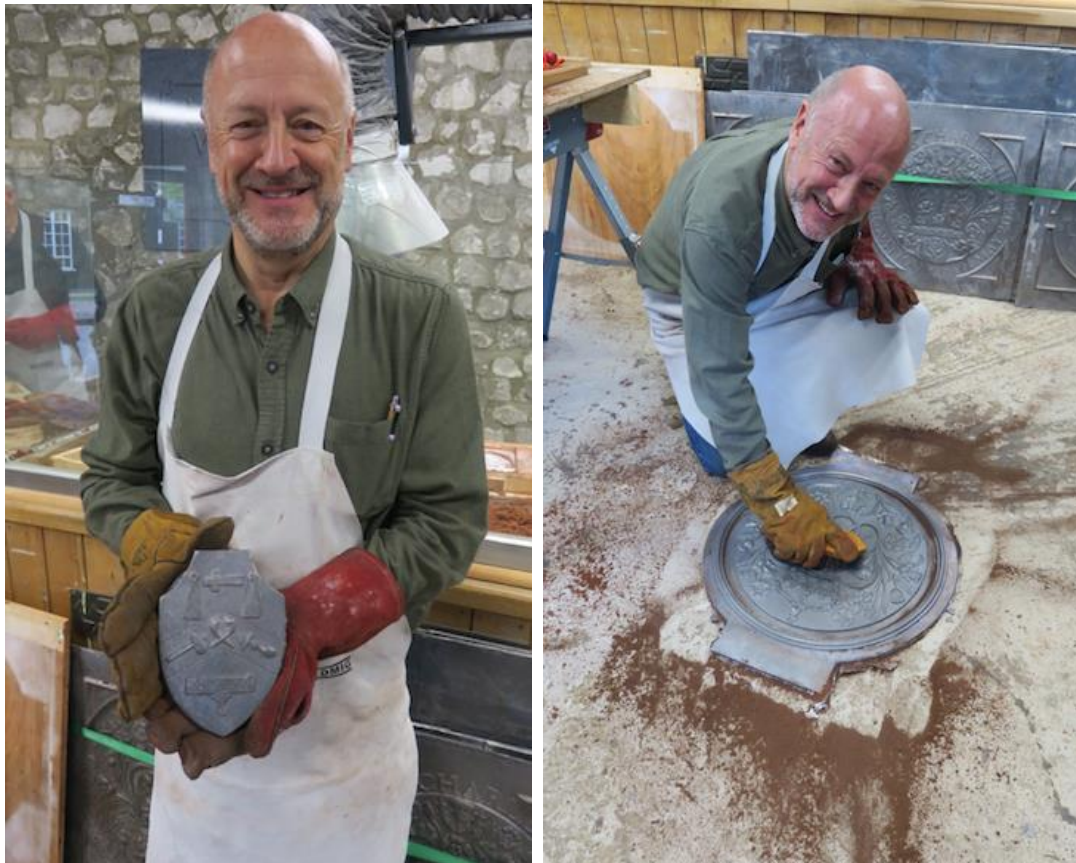
Casting the Coronation Planters at the Plumbers Museum Workshop Trust, Amberley
